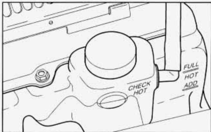
The coolant level should be at least up to the ADD mark. If it isn't, you may have a leak in the radiator hoses, heater hoses, radiator, water pump or somewhere else in the cooling system.
