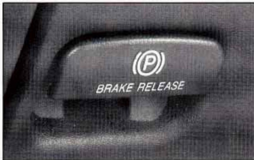
Pull the BRAKE RELEASE lever. It is located on the bottom of the instrument panel on the driver's side.
